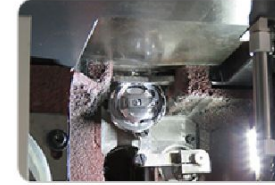
Using 2 times big hook to improve working efficiency and reduce the time of replacing bobbin
