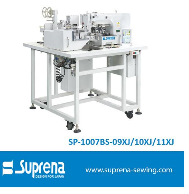
Full automatic process: Auto feeding, cutting, stitching and collecting can be done by one button .
